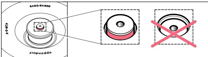
The loose positioning of the upper shell is intentional and aids in self-centering.
