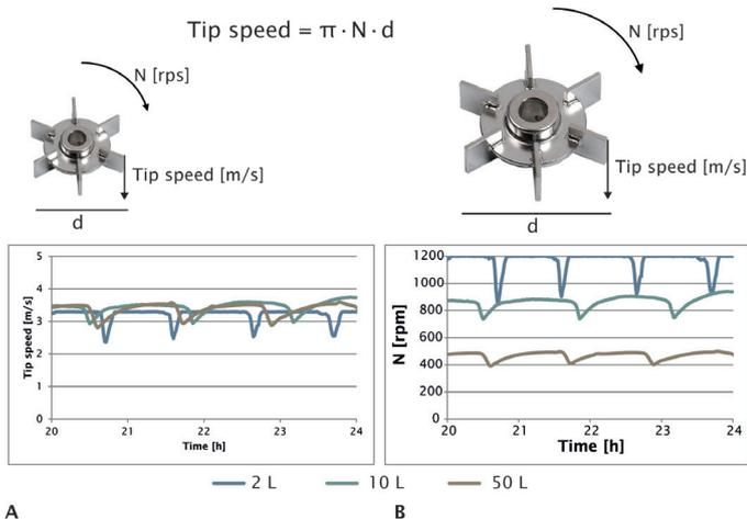
**Figure 3:** Comparison of turbine tip speed and stirring speeds when controlling the dissolved oxygen concentration at 10% in fermentations at three different scales
