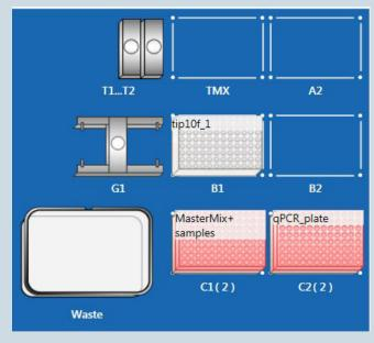
Figure 1: epMotion 5073I worktable for qPCR setup
