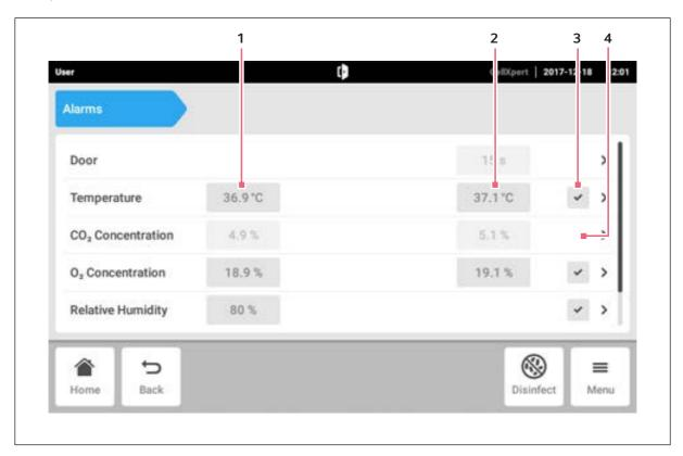
Fig. 8-6: Overview with device alarms, warning limits and alarm limits
