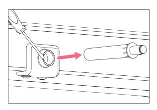
1. Remove the door damper with the flat head screwdriver.
