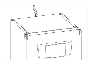
4. Click the two parts of the magnetic safety latch together.
