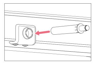
1. Insert the longer and thicker part of the door damper into the holder.
