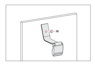
3. Attach the other part of the safety latch and a washer to the wall. The screw must have a pullout strength of at least 250 N (25 kg).
