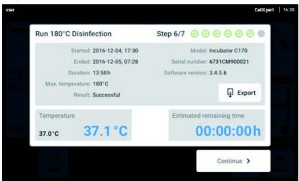
Fig. 10-9: Display of the result of the high-temperature disinfection after achieving the target temperature 8. Follow the instructions on the touch screen.
