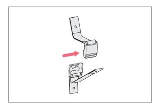
1. Disconnect the upper and the lower part of the magnetic safety latch by pushing them aside from each other.
