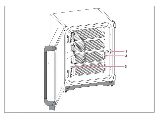
Fig. 3-6: Inner door with 4 door segments
