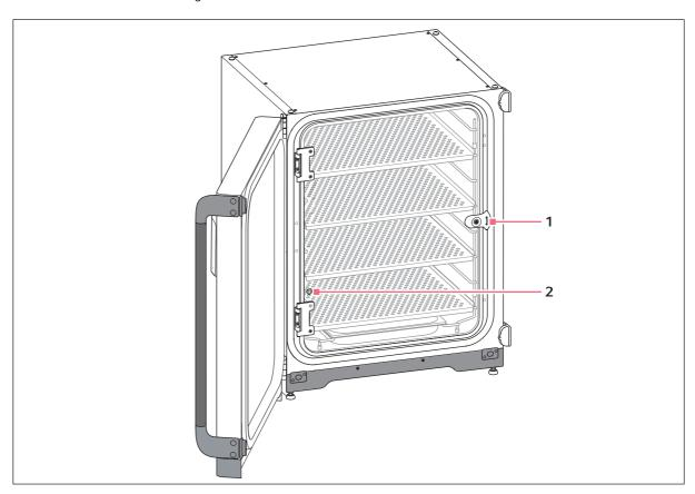
Fig. 3-5: Non-segmented inner door
