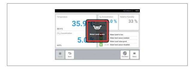
A hint appears on the screen, when the water level falls below 0.5 L. The hint recurs every 15 minutes until the water tray is refilled. The alarm function is ready for action 2 hours after the door has been closed and 1 hour after the device has been switched on.
