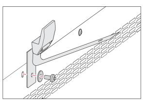
2. To attach the lower part of the safety latch to the top side of the incubator, use the spare part screw M4x8, Torx 20, and a washer.
