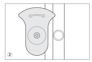
Fig. 5-2: Inner door latch with magnet
