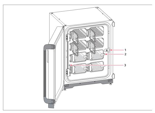
Fig. 3-7: Inner door with 8 door segments
