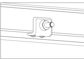
2. Press the door damper into the holder until it stops.
