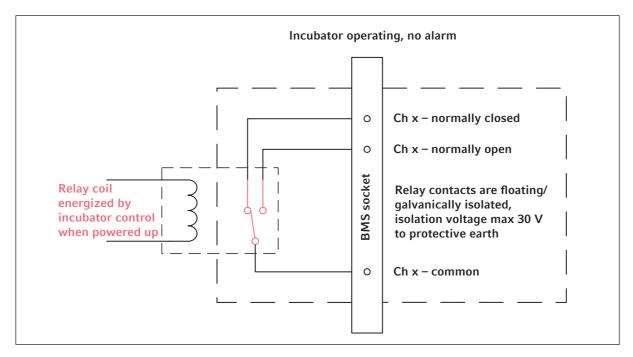
Fig. 4-4: Incubator operating without alarm
