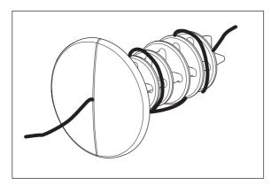
Fig. 5-3: Wire wrapped around the blind plug
