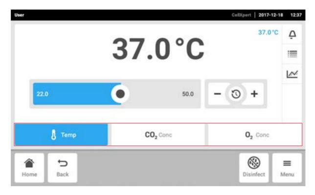
To switch to another function, tap on the symbol of the required function. The active function is highlighted in blue.
