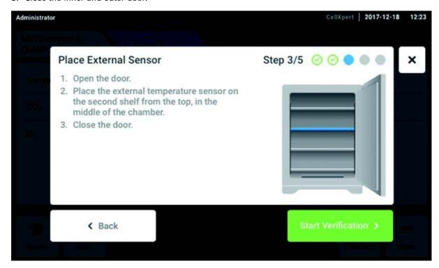
Fig. 10-3: Placement of the external temperature sensor
