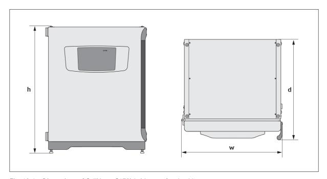
Fig. 13-1: Dimensions of CellXpert C170i (without safety latch)
