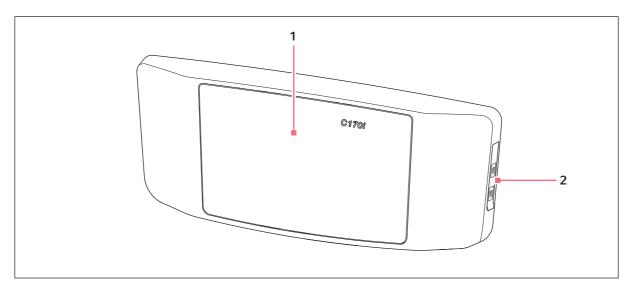
Fig. 3-2: CellXpert C170i: Control unit
