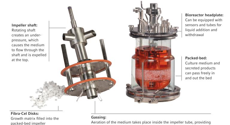
a bubble-free aeration in and around the packed-bed, which is
